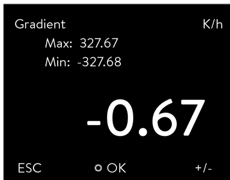
Fig. 73: Entering the gradient
